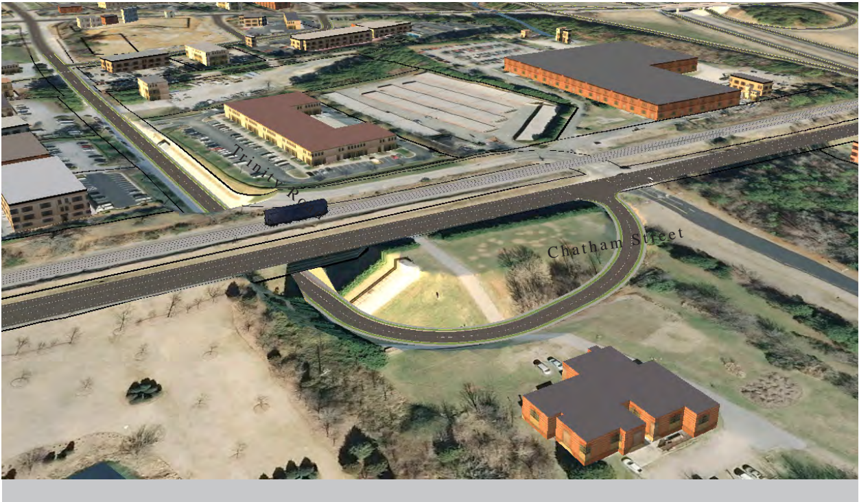
Trinity Road bridge over the railroad at new crossing location with loop ramp to Chatham Street
