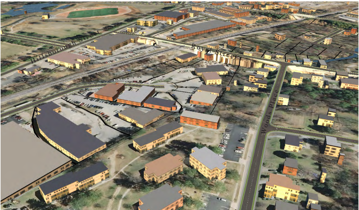
Royal Street bridge over the railroad, connecting directly to Hillsborough Street, add a new connector from Beryl Road to Royal Street and close Beryl Road crossing
