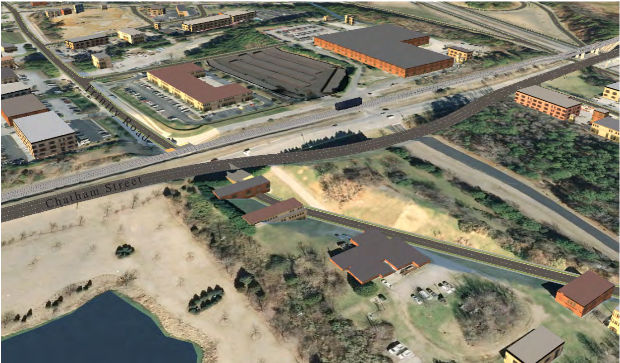
Railroad bridge over Trinity Road at new crossing location, shifting the Maynard Road/Chatham Street intersection to outside of the 200' railroad corridor
