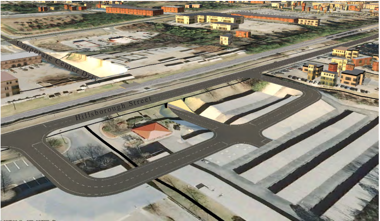
Railroad bridge over Corporate Center Drive extension, extended to Hillsborough Street, connecting extension to Hillsborough Street with loop ramp
