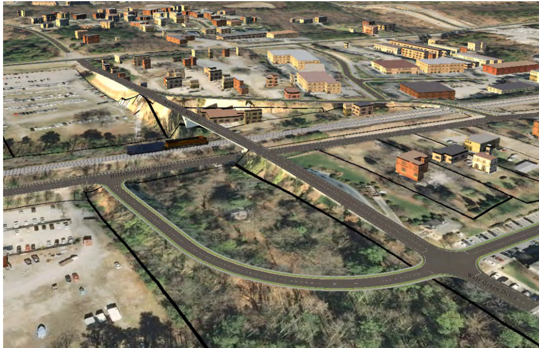
Nowell Road bridge over the railroad and Hillsborough Street with loop extension ramp to Hillsborough Street
