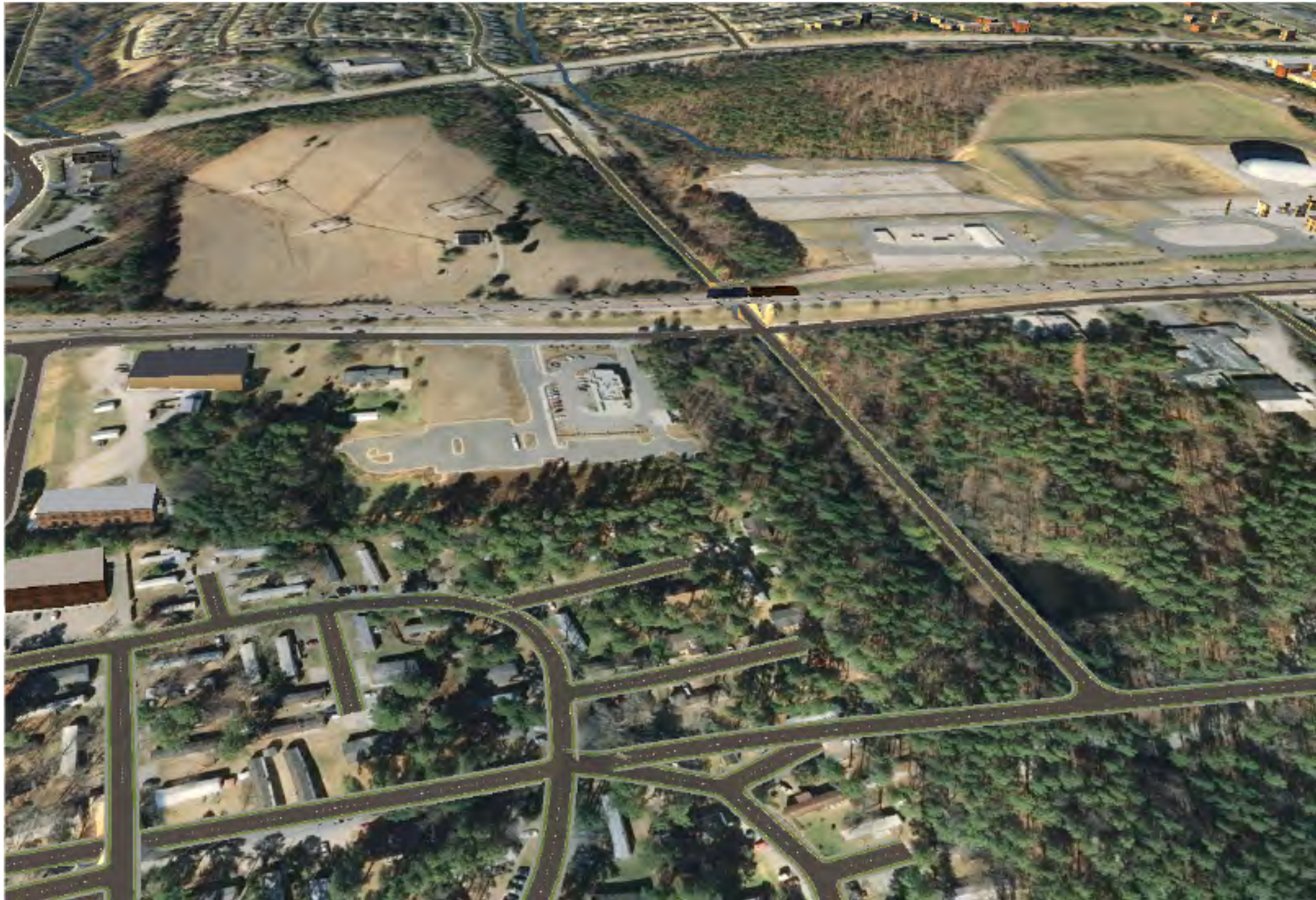
New crossing under the railroad, located between NE Maynard Road and Trinity Road. New road would extend north to Chapel Hill Road and future east-west connector to Cary Towne Boulevard extension
