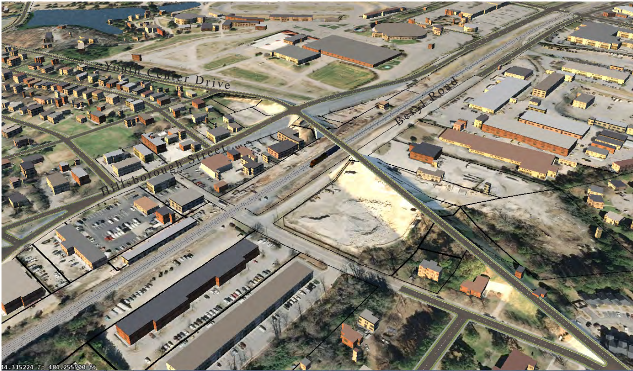
Realignment of Powell Drive to connect with Youth Center Drive with a bridge over the railroad
