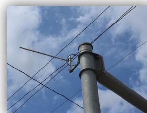
Figure 2.4: Yagi antenna for 900 MHz wireless communications
