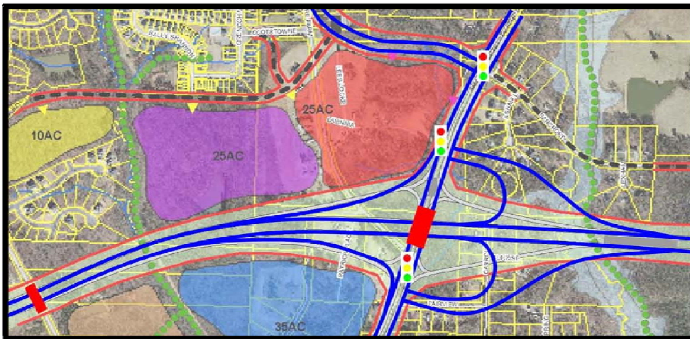
Figure 4. Concept 6: Half Clover Interchange with 2 Ramps at Holly Springs Road
