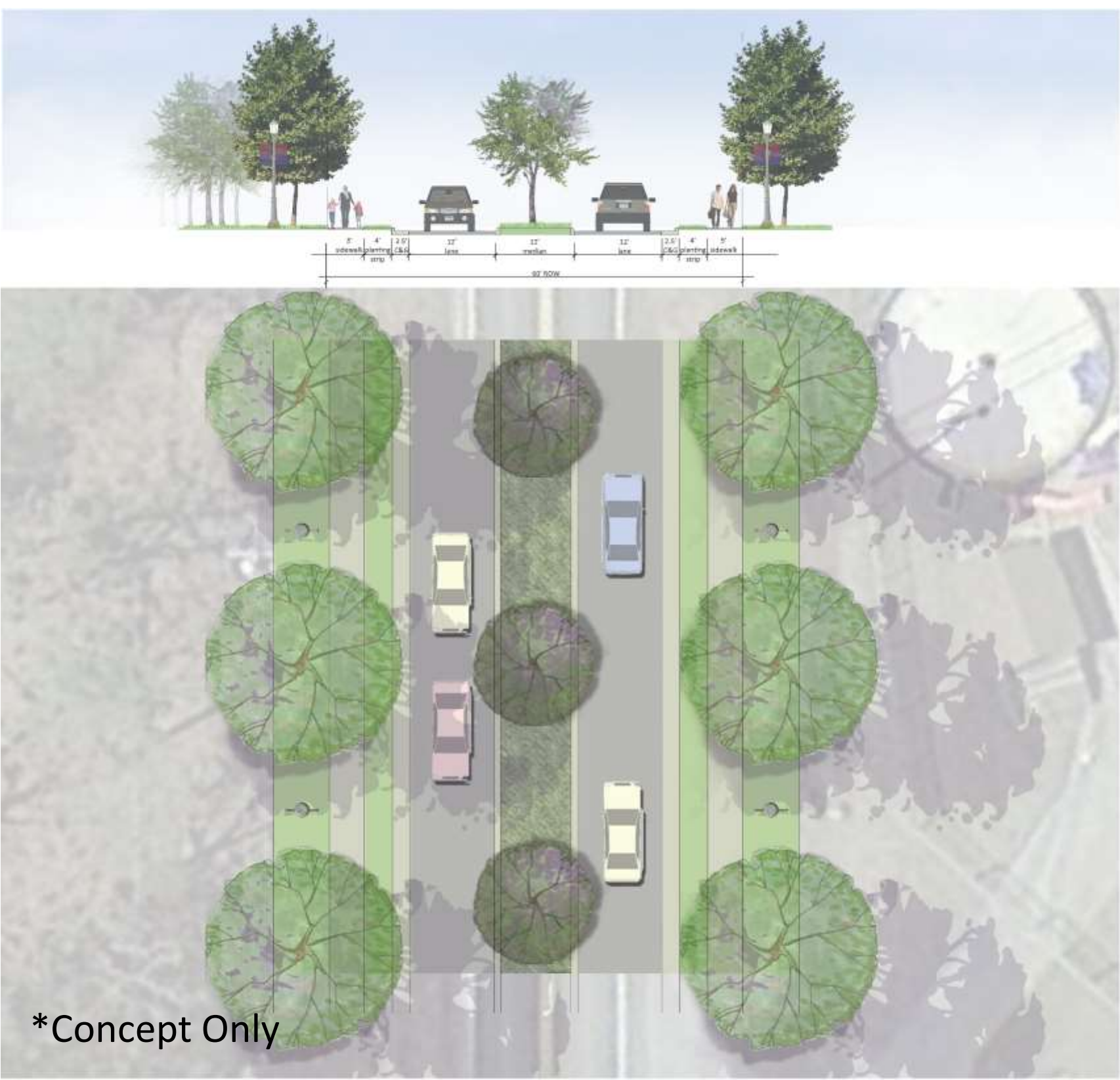
Two-Lane with Median Cross-Section areas without many driveways could have a planted median instead of a center turn lane
