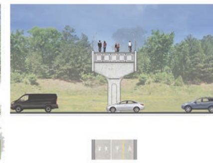
16' Separated Use Bridge (Min. 17' Vertical Clearance over I-40)
