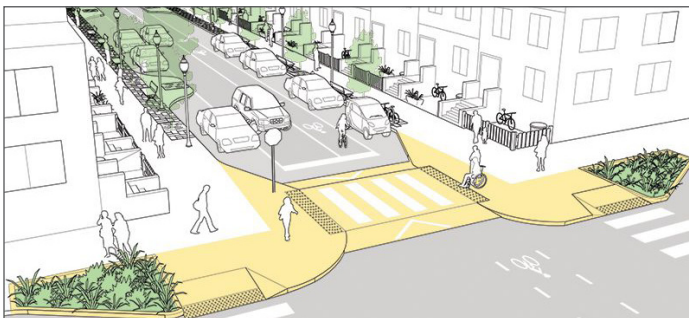
Example of a raised crossing. Source: NACTO
