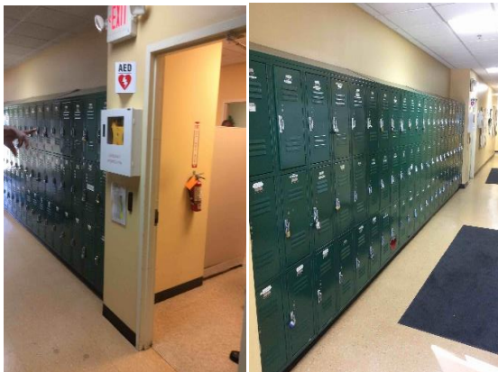
Drivers' lockers are located in the main egress path
