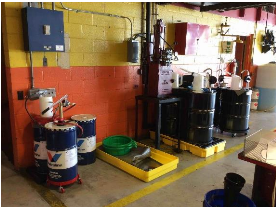
Fluids are stored in the maintenance shop area via drums instead of utilizing bulk storage tanks in a secure lube room
