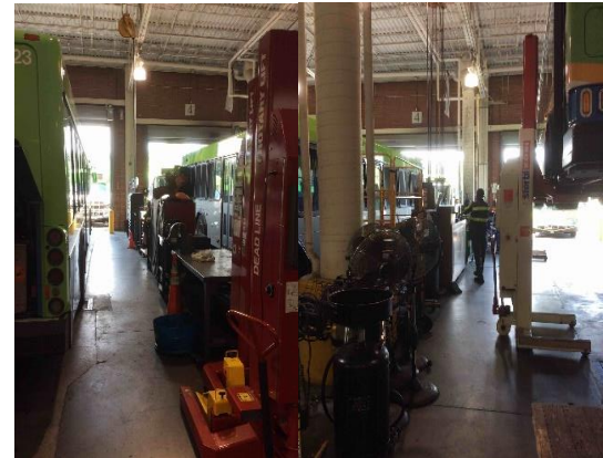
Toolboxes and shop equipment are stored between repair bays because of the lack of equipment storage space
