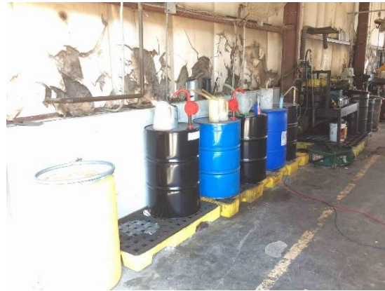
Bulk fluid is stored using 55 gallon drums along the back wall of the facility.
