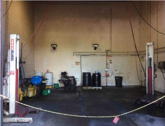
The steam room utilizes two portable lifts to lift only one end of the bus instead of a drive-on type lift
