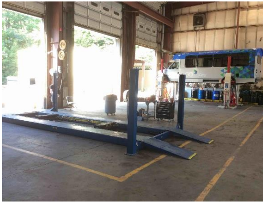
Surface mounted and portable lifts are used to maintain and service the buses.
