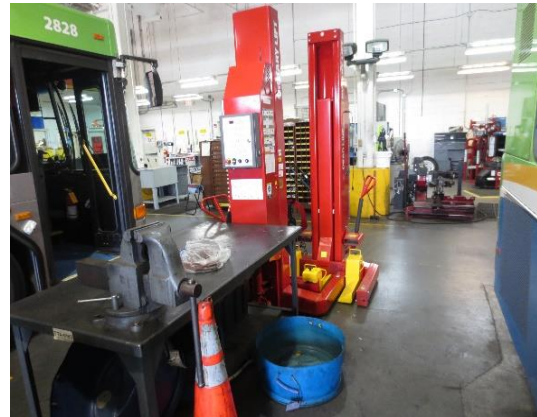
Work benches/workstations are between bays restricting the circulation around buses when serviced
