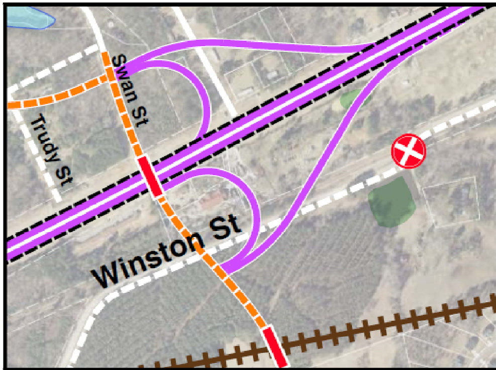
Figure 4-9. Partial Cloverleaf Interchange with Loops in SW and SE Quadrant Recommended for Interchange in Northern Franklin County
