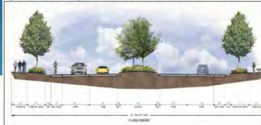
Figure 24: Major Thoroughfare, 4 Lane Divided Cross-Section
