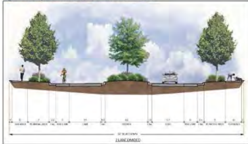
Figure 26: Major Collector, 2 Lane Divided Cross-Section
