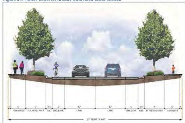
Figure 29: Minor Collector, 2 Lane Undivided Cross-Section
