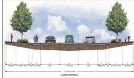
Figure 27: Major Collector, 3 Lane Undivided Cross-Section
