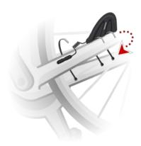
2. Attach the spoke magnet to one of the spokes on your bike. The magnet should face the chainstay where you attached the chainstay sensor.
