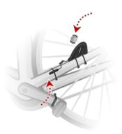
Once you have adjusted the sensors to the right position, tighten the cable ties so they are held securely in place.
