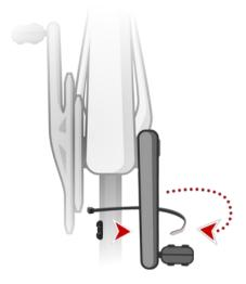
**Tip**: Make sure the different parts of the Cadence/Speed Sensor are lined up correctly on your bike. The spoke magnet should pass the main body of the chainstay sensor and the crank arm magnet should pass the tip of the sensor.
