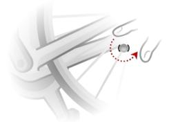
3. Adjust the position of the spoke magnet and the chainstay sensor so that when the wheel turns the spoke magnet passes the tip of the main body of the chainstay sensor.
