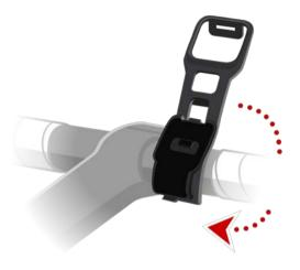
3. Use the clip on the bottom of the holder to attach the handlebar strap to it. The strap should now be attached securely around the handlebar.
