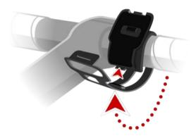
4. Remove your watch from the wrist strap and place it in the holder. Make sure it clips securely into place.
